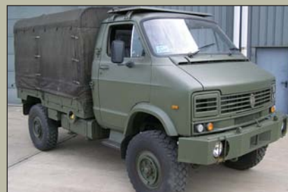
LReynolds Boughton RB 44 Truck Cab Pickup R.H.D , Permanent 4x4, 5 speed g/box, hi/lo box differential Lock, power steering, carries 2250 kgs, Perkins Phaser 110T T/Diesel engine, Mileage from 37,000, Guide price from £3,750 (10 Available)
